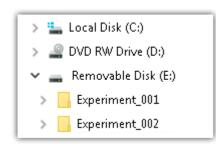
To perform formatting of a storage medium via the Windows-Explorer 24, navigate to the desired storage medium. Run the formatting by means of the context menu, for example.
