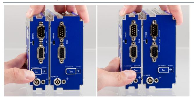
3. Switch the locking slider in "CONNECT"-position. The modules are now electrically connected and mechanically saved. In order to separate the module, switch the locking slider back into the "DISCONNECT"-position.
