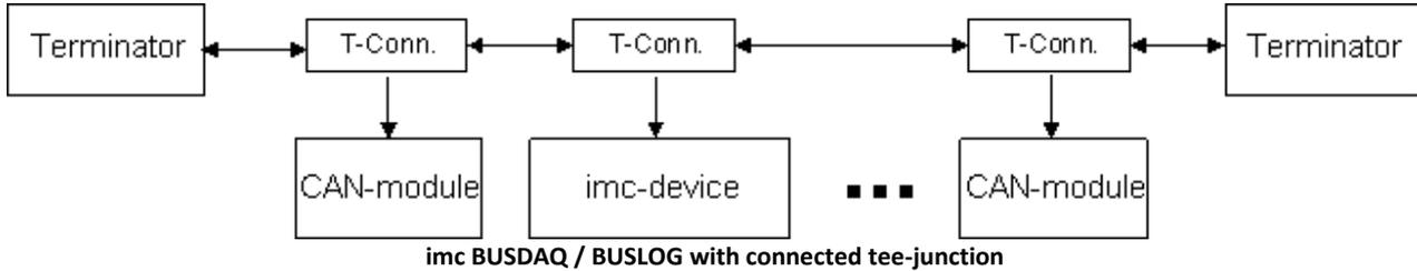
Note that for a transfer rate of 1 Mbit/s to the CAN-Bus the stub line of a tee-junction may only be up to 30 cm long. In general, the wiring within imc BUSDAQ / BUSLOG is already 30 cm long. Therefore if an external tee-junction is connected, the junction must be connected straight into the terminal.
