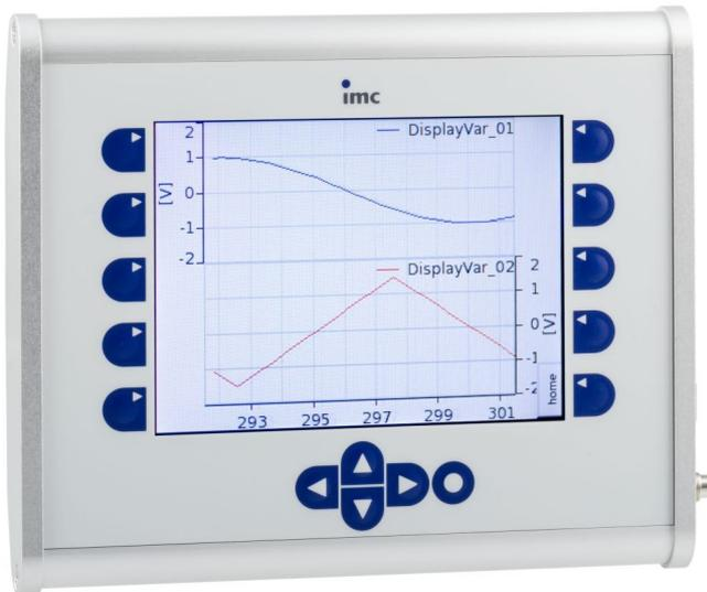
The optional display screen enables interaction between the user and a running measurement process by posting read-outs of system states and allowing parameter adjustments via the membrane touch panel.
