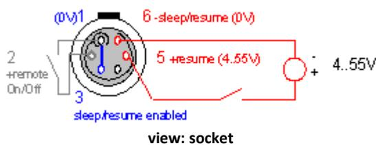
Pins 1 and 3 are connected to activate the Sleep/Resume mode.
