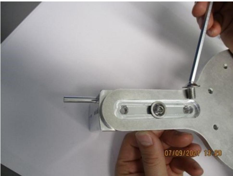
Use the three slotted holes to set the inner radius of your steering wheel as well as possible; the fine adjustment is then made directly on the steering wheel.
