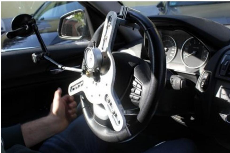
Turn the steering wheel by 360°. Using the dial gauge, you see what deviation you will get in the individual spoke of the steering wheel fastening. You must compensate for this deviation as well as possible via the slotted holes. A deviation of  $\pm 0.5$  mm will be acceptable.
