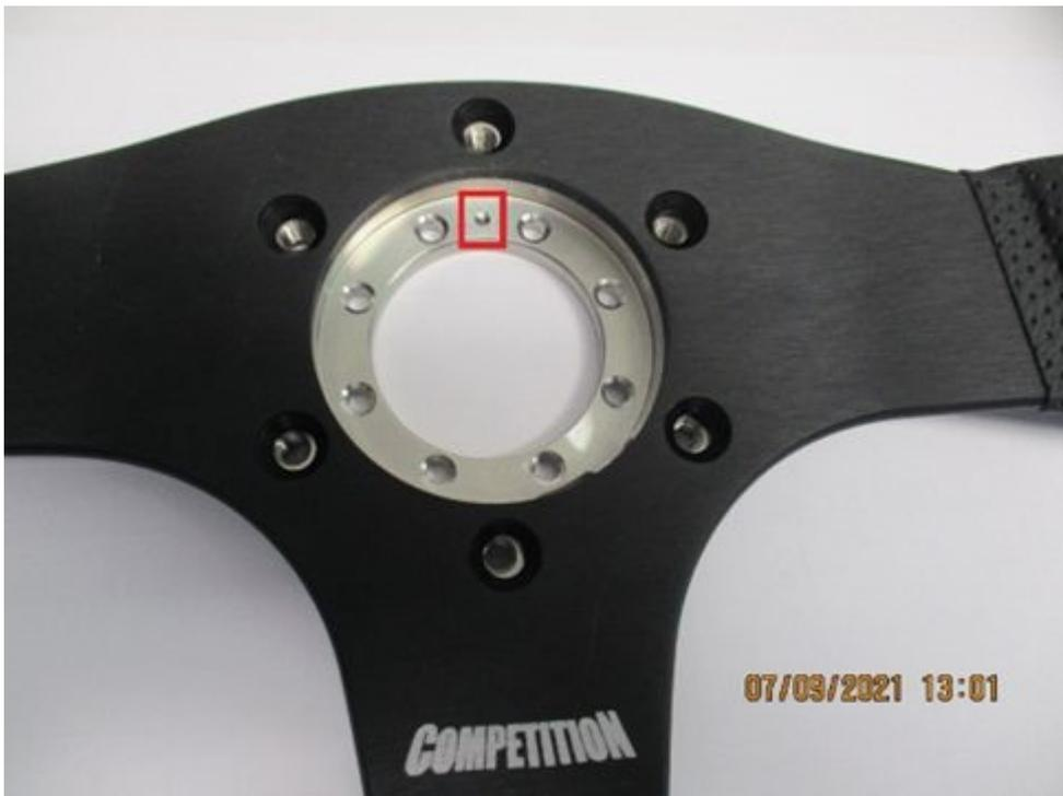
Mount the CLS<sup>x</sup> steering sensor to the sports steering wheel adapter. The upper side of the CLS<sup>x</sup> steering sensor faces the sports steering wheel. Follow the instructions below for the sequence and tightening torque of the screws.
