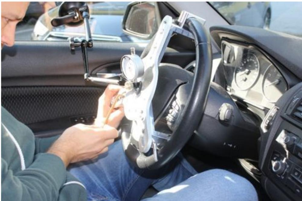
Once the steering wheel fastening is centered, fix it to the remaining spokes with the brackets.
