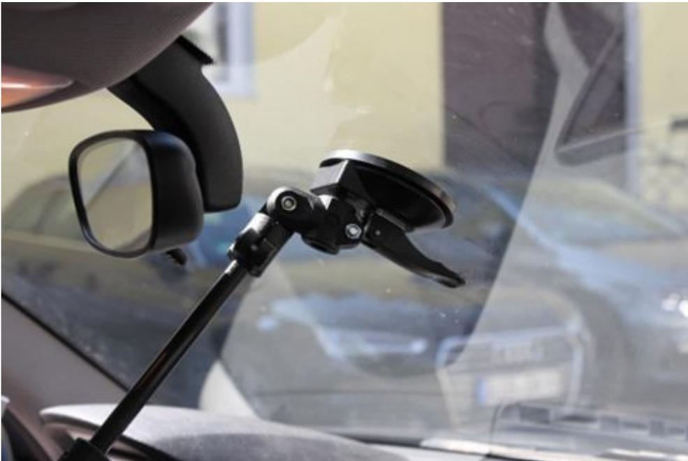
Lead the CLS<sup>x</sup> sensor cable out along the carbon rod and fasten it with adhesive tape or cable tie.
