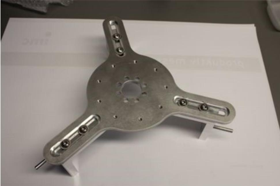
Depending on your wanted distance between the steering wheel fastening and the vehicle steering wheel, you can choose three predefined distances. Here you need to attach lateral positioning pins (see red marking in the picture below).
