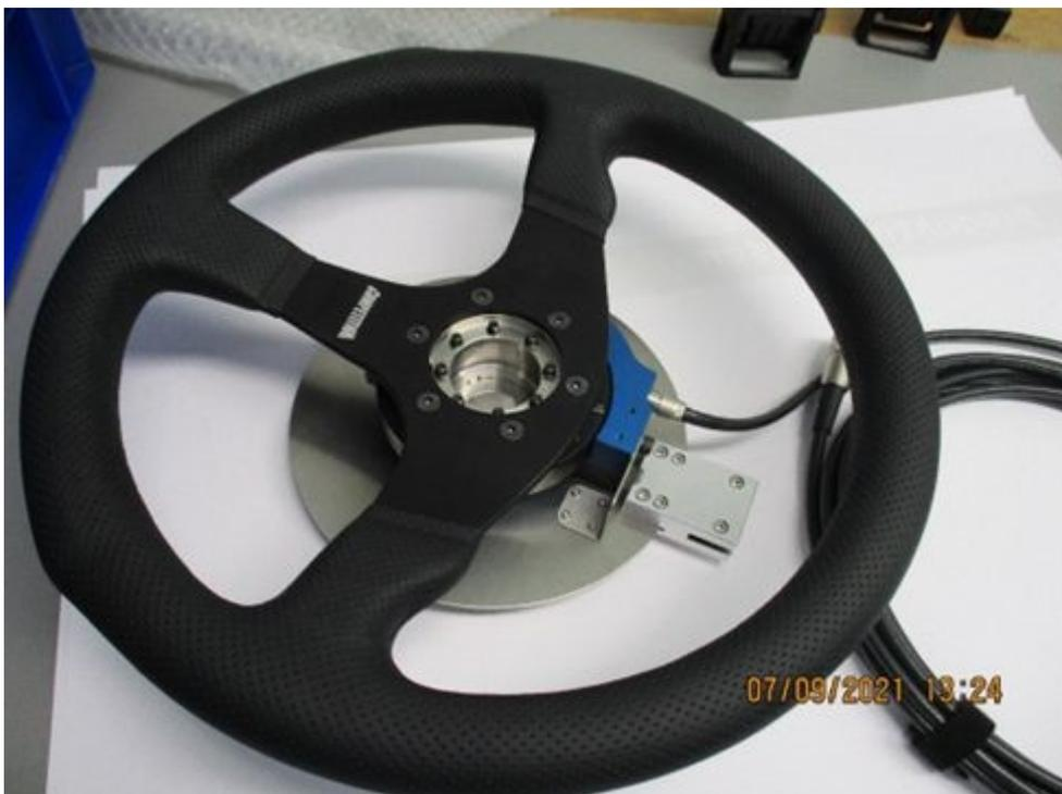
The steering wheel fastening is designed for variable steering wheel diameters. It can be individually adjusted via slotted holes.
