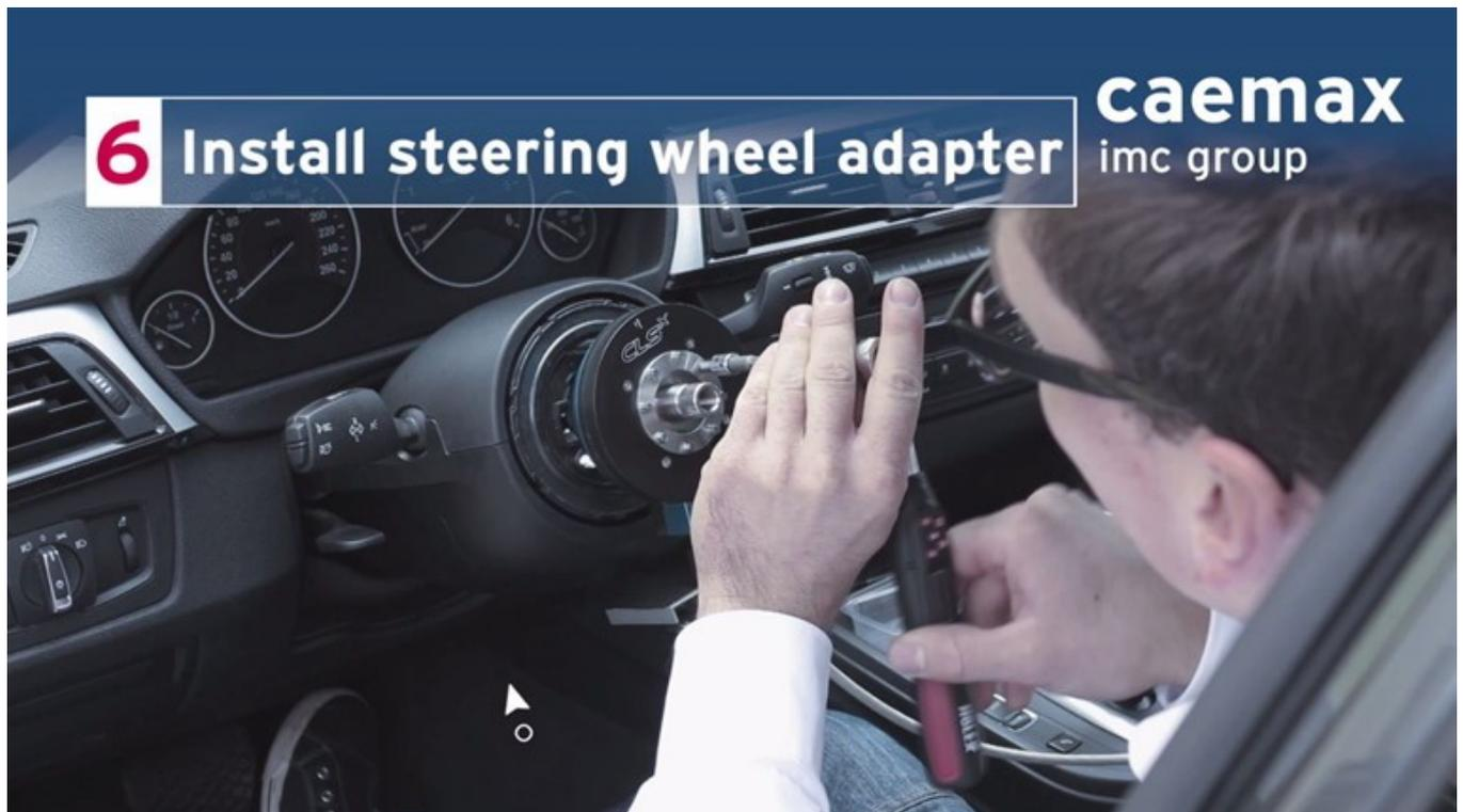
Now please tighten the 8 screws with the final torque of 6.0 Nm in the order shown in the picture below.
