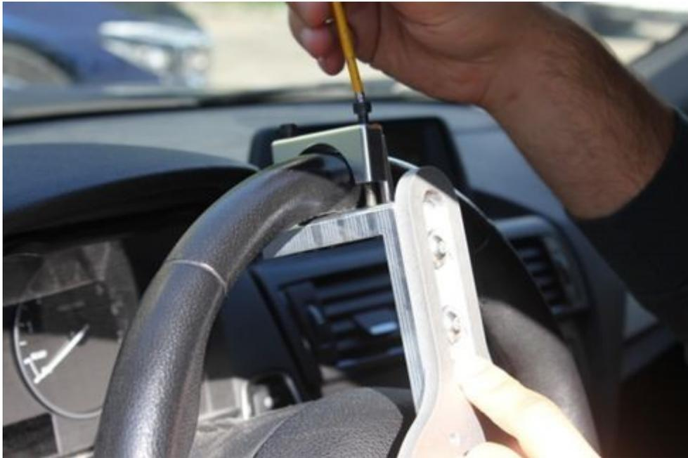
In the next step the exact centering of the assembly will follow. To do this, install the dial gauge. Attach it to the inside of the side window with the suction cup. The sensor of the dial gauge must rest on the fit in the center of the steering wheel fastening.
