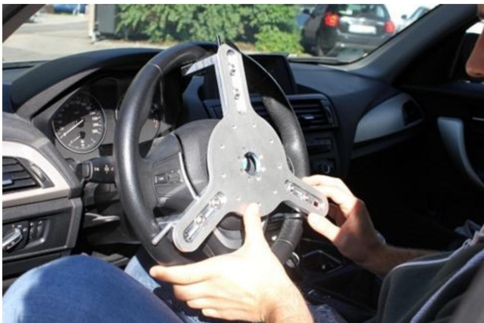
Fix the steering wheel fastening on the upper spoke with the bracket.
