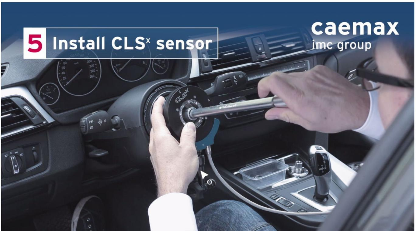
Attach the steering wheel adapter to the CLS<sup>x</sup> steering sensor using the appropriate screws provided.
