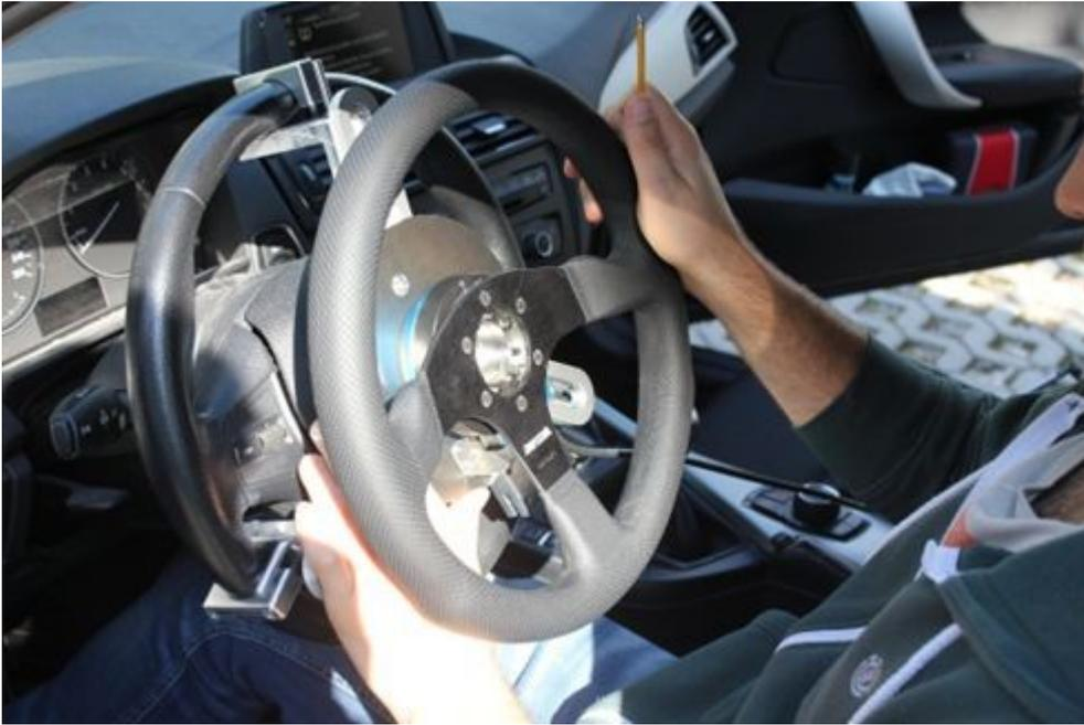
The disc of the torque arm shows a hole (red marking in the picture below). Turn the disc in each case so that it is placed one after the other over the 9 holes for the screws. Fasten the assembly with the 9 DIN 7991 M 6 x 12 screws. Tighten them to hand tightness.
