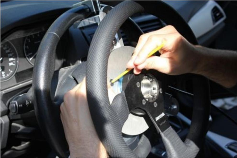
Attach a carbon rod to the torque arm.
