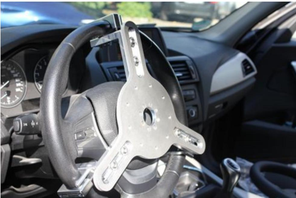
Mount the CLS<sup>x</sup> with the sports steering wheel that you have prepared before on to the TSW adaption.
