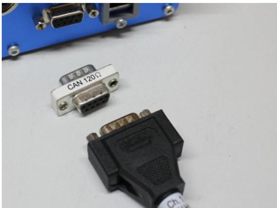
Fig. 6: CAN terminating resistor
