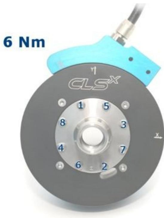
Mount the retaining bracket of the torque arm to the CLS<sup>x</sup> steering sensor. Use the DIN 912 M 5 x 8 cylinder-head screw for this purpose.
