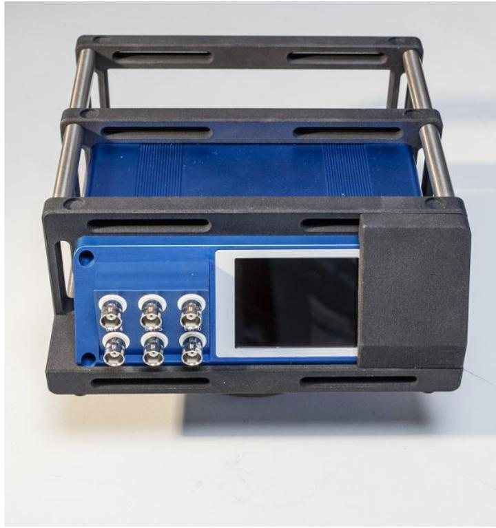
*Fig. 13: CLS-CU mounting frame (example)*
