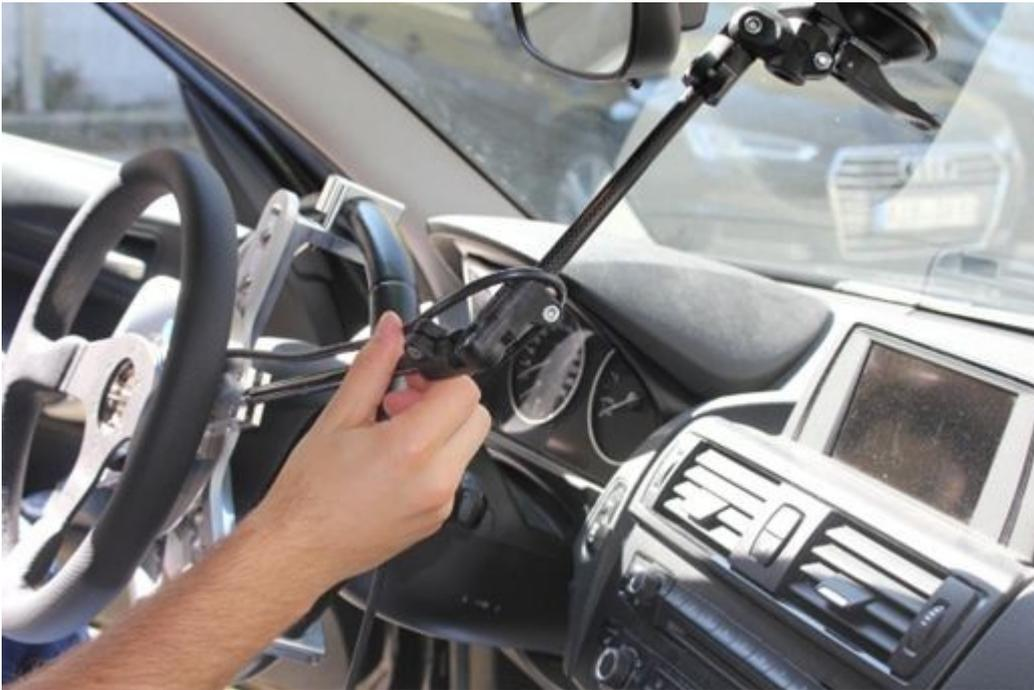
Connect the CLS<sup>x</sup> sensor cable to the sensor input of the CLS<sup>x</sup> control unit (CU).
