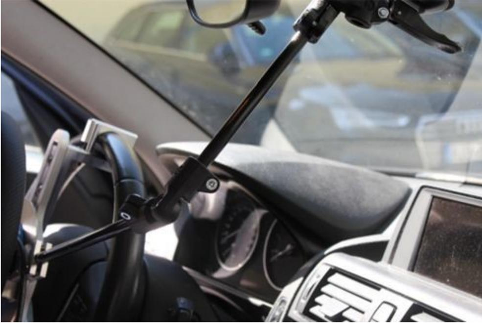
Attach the suction cup mount to the windscreen in a way that your field of vision remains as free as possible, e.g. underneath the rear-view mirror.
