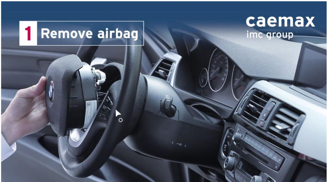
Disconnect the airbag cable connection and remove the airbag completely. To re-establish the steering wheel multimedia cable connection, feed the cable through the CLS<sup>x</sup> steering sensor after disconnecting the connector.
