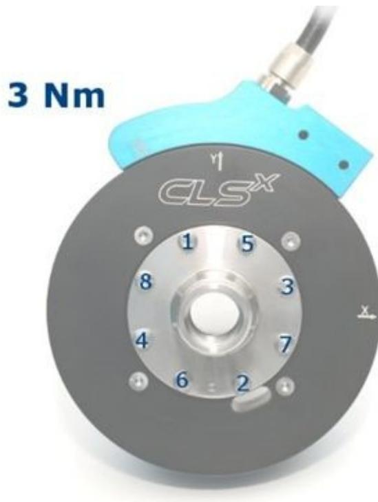
Now tighten all 8 screws with the final torque of 6.0 Nm in the order shown in the picture below.
