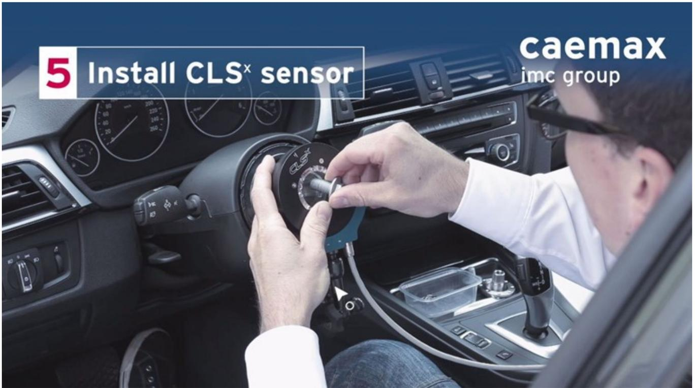
Tighten the central screw according to the vehicle manufacturer's specifications.
