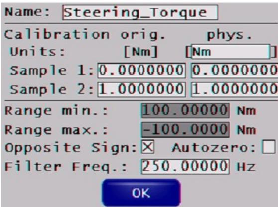
To save these settings permanently, select *Load/Save* and save the current configuration as *DEFAULT.dxp*. Activate *Save* and confirm *Parameters saved!* with *OK*.
