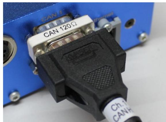
Fig. 7: plugged-in CAN terminating resistor
