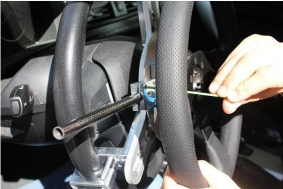
Assemble the mount for the torque arm with the joints and the carbon rods. Adapt this to your requirements. If necessary, you can also shorten the carbon rod. In practice, it has proven useful to first fix the carbon rods with the screws in the joints so that they no longer slip loosely, but remain adjustable.
