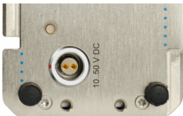
input power supply socket LEMO.1B (female) for a connection with 24 VDC power adaptor (1 guide notch, LEMO.EGG.1B.302)
