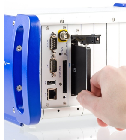
CRC/HDD-FRAME how to insert the SSD
