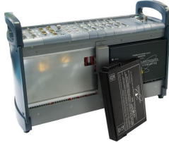
imc CRONOScompact with two Li-ion battery packs The batteries are equipped on the bottom.
