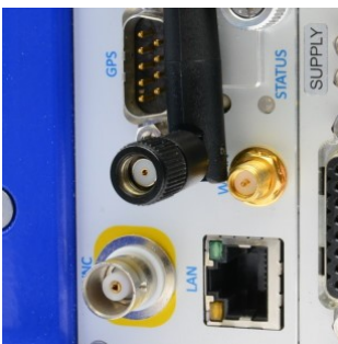
WiFi - antenna with RPSMA (female) connection at your device RPSMA (male)
